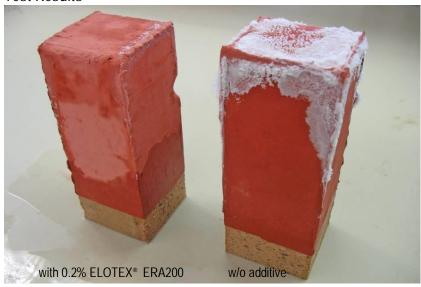
Quick test method for secondary efflorescence. Skim coat is applied on porous clay brick and partially immersed into salt solution for several days.
