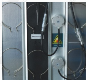
Four sensors monitor UV irradiance
